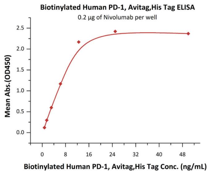
Immobilized Nivolumab at 2 µg/mL (100 µL/well) can bind Biotinylated Human PD-1, Avitag, His Tag (recommended for biopanning) (Cat. No. [PD1-H82E4](#)) with a linear range of 0.8-13 ng/mL (QC tested).
